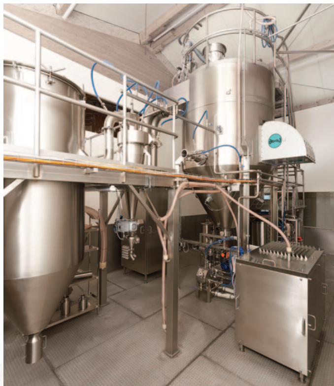
Pilot-scale spray dryer in the VetterTec Test Centre – bridging the gap between lab results and industrial production.
